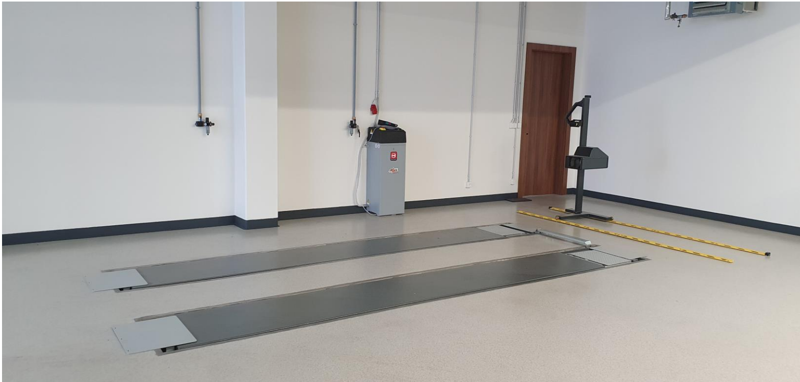
SF6354I Electro-hydraulic scissor lift, Capacity 3500 kg With built-in play detector
