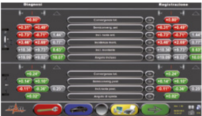
屏幕上同时显示汇总的诊断数据并进行比较 Summary and comparison of diagnosis/repair values on a single screen.
